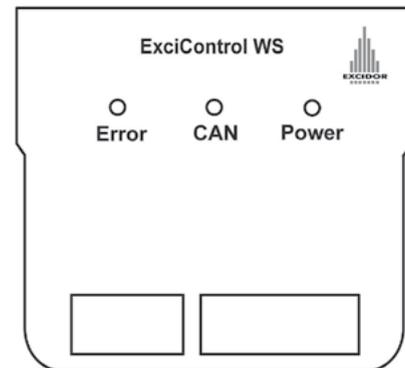
Indicator lights on the main controller, Error, CAN and Power.
